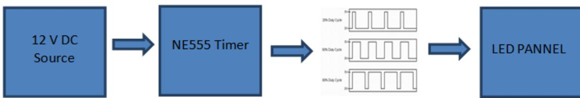
The DC source is given to the NE555 timer. NE555 timer is used to generate the PWM signal. The width of the PWM signal always depends on the duty cycle, so we can vary the duty cycle through NE555, if we can vary duty cycle we can generate the pulse with various width.so we use timer to generate the PWM to dimmer the LED or increase brightness of the LED.
